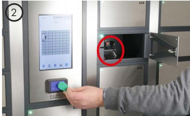
The RFID recognition of the locker system recognises the **green chip** and opens the employee's individual locker. Stored inside are his work equipment and a **red chip**.
